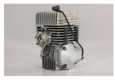
**KT Ignition:** The standard KT 100S (unmodified) ignition to be used, the fitting of the following modules as an alternative to the standard KT 100S ignition module is permissible: Yamaha, Victa, Atom, Delta, Wei/Shieh, Sig, Nova, PRD, and TCI are permitted. Ignition key is a non-tech item. The rotor must be OEM with no modifications. The rotor outside diameter may be cleaned or lightly sanded but no additional machining is allowed.
